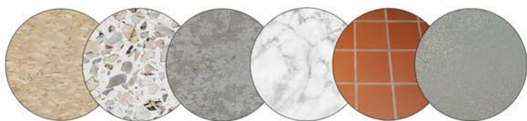
VCT TERRAZZO CONCRETE MARBLE QUARRY TILE POURED EPOXY
